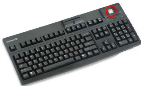
Wireless keyboard with integrated sensor (upper right corner)
