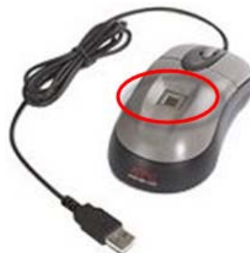
USB mouse with integrated sensor
